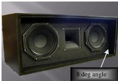
**OD 8211 BC:** This model has an internal 8 deg frontal angle. Please observe top and bottom factory labeling when mounting. Proper positioning has speaker firing upward (“top” label on top side), if near ground level, and downward (“top” label on underside) if placed 5 ft or greater above the ground.
